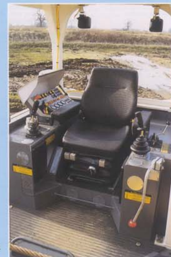
The pipe layer can also be equipped both with a canopy and a fully enclosed operator's cab.
