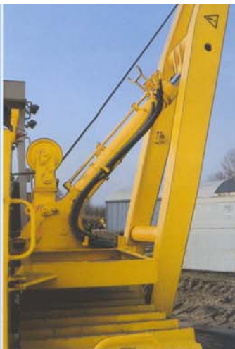
The boom can be adjusted precisely and without sudden jerks with a hydraulic cylinder.
